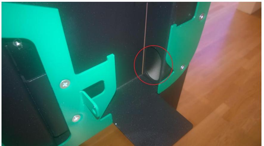
Figure 14: Exit cable hole located behind the position where the charging station will be attached to the standing pole
