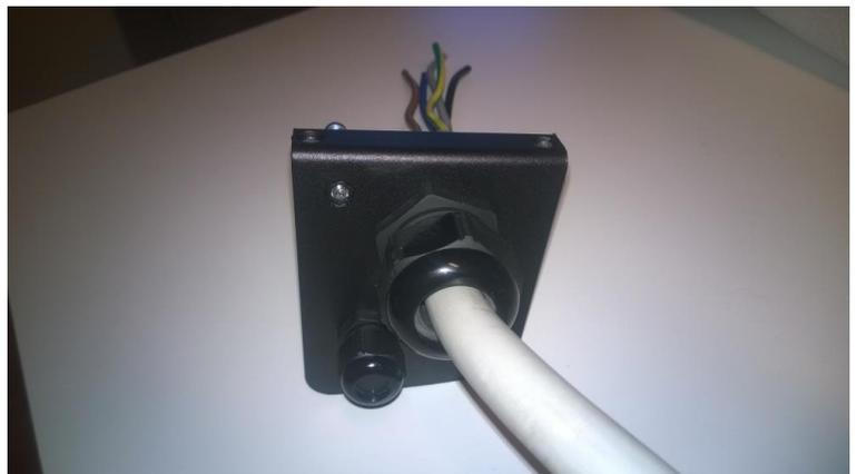
Figure 40: Power supply cable pulled through the gland – front view
