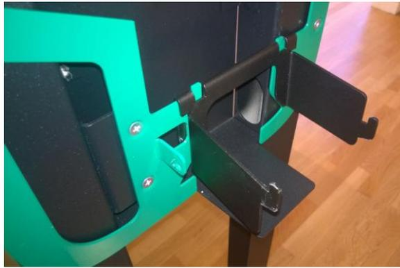
Figure 22: Wall mounting bracket installed on mounting pole with temporarily attached installation holder
