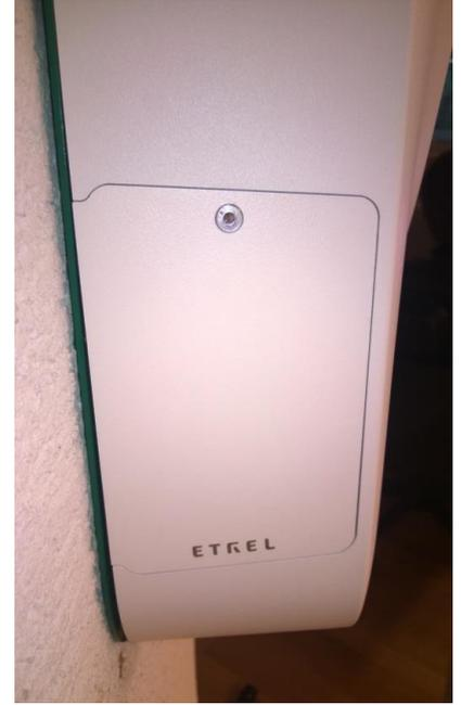
Figure 72: Secure maintenance doors to the enclosure
