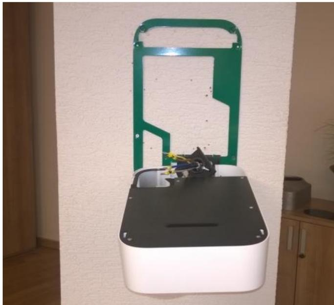
Figure 50: Charging station mounted on the holder - front view
