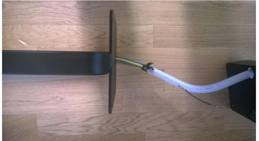
Figure 16: Pulling the cable through the column with leading cable and duct-tape.
