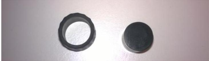
Figure 46: Removed filler from the gland rubber
