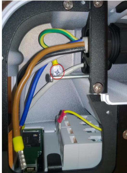
Figure 55: Ground wire secured to the enclosure using the screw
