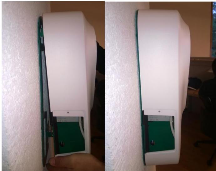
Figure 69: Attach the charging station to the top hooks of the mounting bracket and push it to the wall
