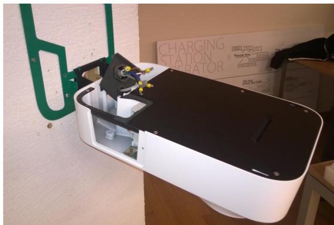
Figure 51: Charging station mounted on the holder - side view
