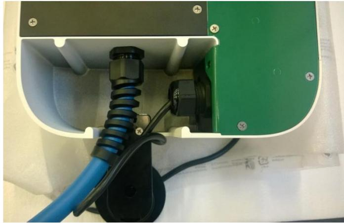
Figure 66: Installed metallic cable holder
