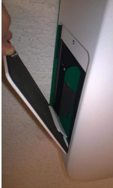
Figure 71: Attach the side doors to the enclosure
