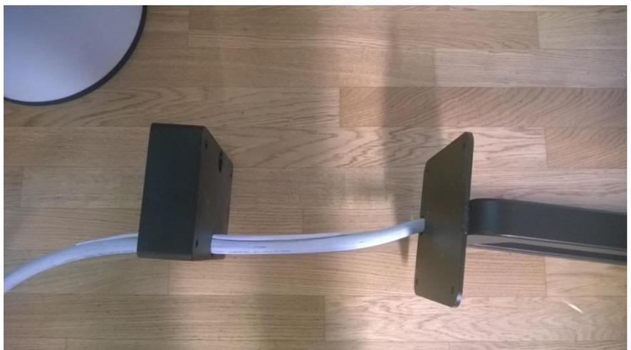
Figure 15: Cables pulled from the top of anchoring structure and through the column hole in the bottom
