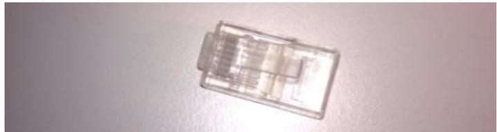
Figure 48: UTP cable plug
