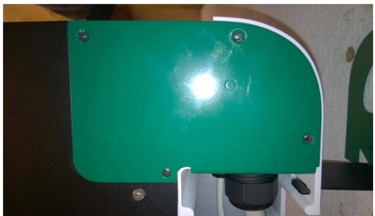
Figure 61: Secure the green back-maintenance cover with screws
