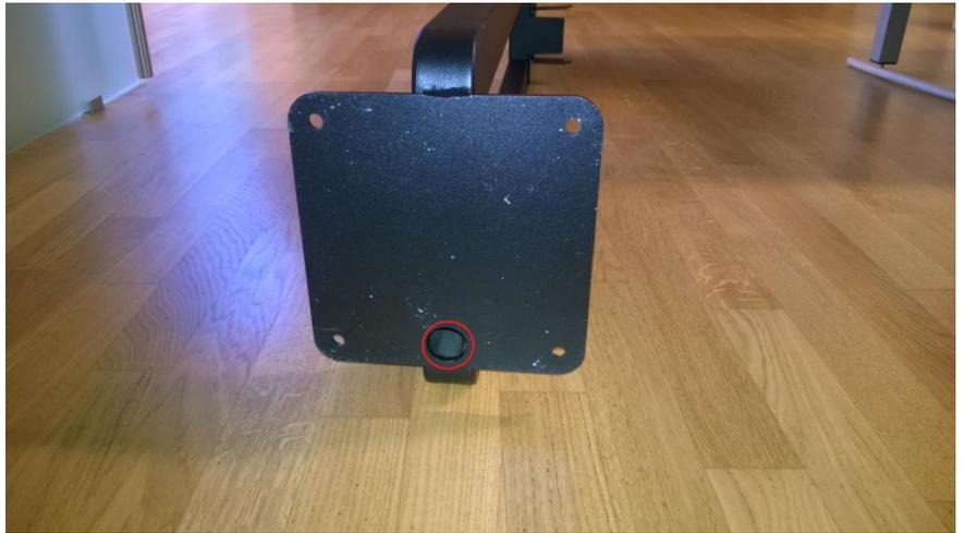
Figure 13: Column hole on the base of standing pole where cables can be inserted from anchoring structure
