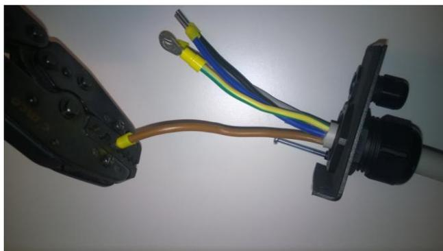
Figure 44: Squeezing the ferrules of the wiring
