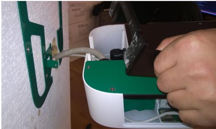
Figure 63: Installation holder is removed
